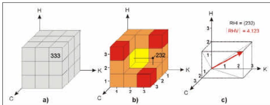
**Figure 4.** The three-dimensional matrix  $ckh$ , used for rockfall hazard assessment. (a) General definition of the positional Rockfall Hazard Index, RHI; (b) splitted matrix cube with ranked RHI values; (c) Rockfall Hazard Vector (RHV) concept.
