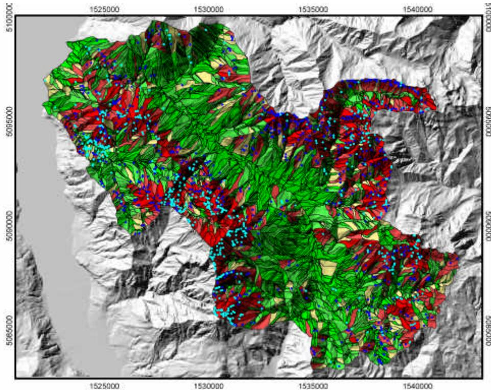
**Figure 3.** Predictive map of debris-flow source area based on a multivariate model that incorporates geological, morphological and land-use factors of slope units.
