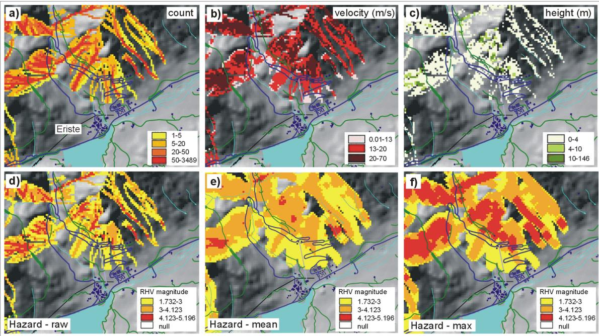
**Figure 3.** Close-up of the rockfall model in the Eriste area: a) rockfall count raster map; b) maximum computed velocity raster map; c) maximum computed height raster map. Hazard maps obtained through the proposed methodology: d) raw map, directly computed; e) map smoothed by the mean value (50 m neighbourhood); f) map smoothed by the maximum value (50 m neighbourhood).
